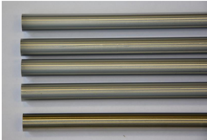
Cr coated ZIRLO cladding tubes
