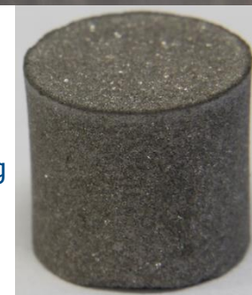
U_3Si_2 pelleting via arc melting and conventional sintering at NNL
